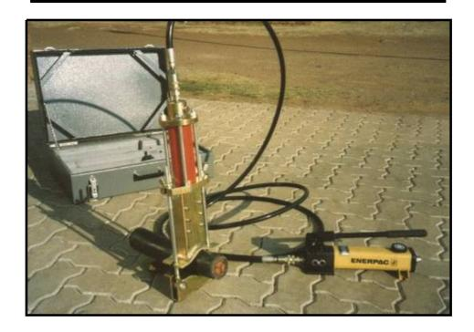
The cable spiking tool is designed and developed by CCE. The spiking tool is totally hydraulic in operation and does not require cartridges or a license to operate. Our product has been developed for use under all conditions and through extensive testing meets all required safety precautions.
